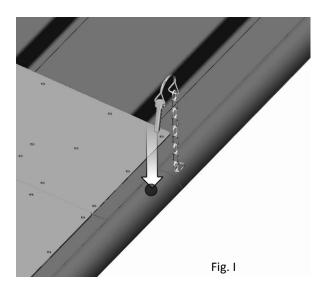
Tighten the central hook (fig. L).
